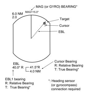
Figure 2-6 Measuring Bearing by the EBL and Cursor
